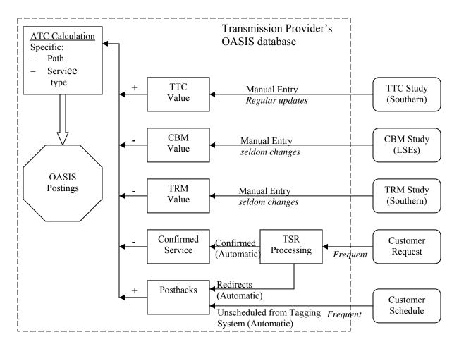
This process flow diagram illustrates the various steps through which a single ATC (based upon specific factors) is calculated. Similar ATC calculations are performed for each path, service type, and time period and will generally result in different ATC values specific to those factors.
