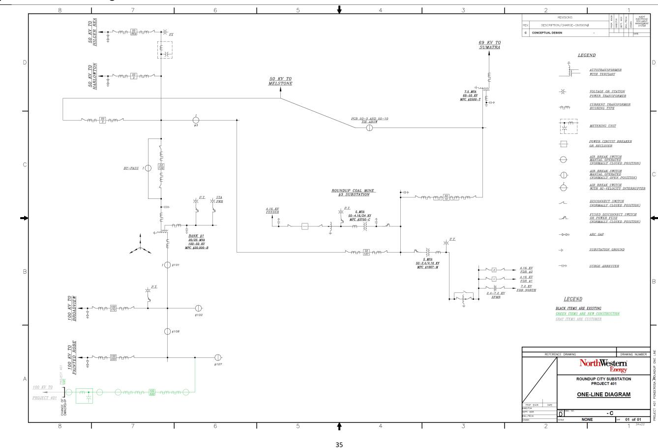
Appendix 1: One-Line Diagram of the interconnection substation
