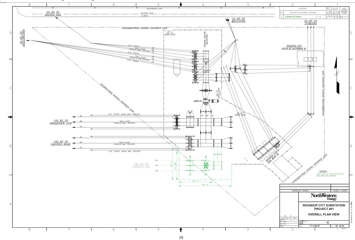
Appendix 2: General Arrangement Diagram of the Interconnection Substation
