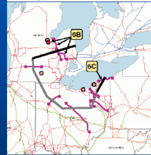
Figure 5.8. Michigan Lines Trip and Ohio Separates from Pennsylvania, 16:10:36 to 16:10:38.6 EDT
