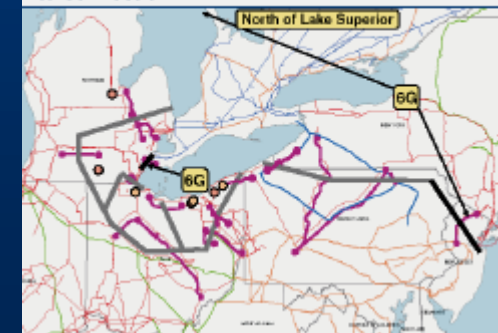
Figure 5.12. Northeast Disconnects from Eastern Interconnection
