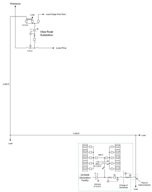
Figure 1: System One Line Diagram
