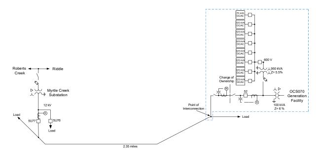
Figure 1: System One Line Diagram
